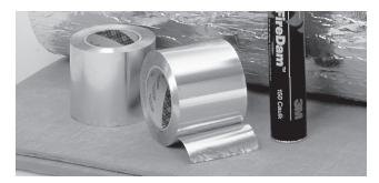
3M Interam Tape T-49 is an adhesive-backed aluminum foil tape designed to seal the cut edges of 3M Fire Barrier duct wrap and interam mats to complete the total encapsulation.
