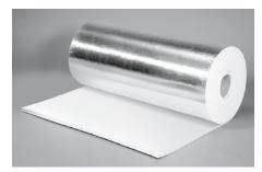
This endothermic wrap is designed to block heat penetration by chemically absorbing heat energy. When exposed to high temperatures, it keeps heat out by releasing chemically bound water to cool the outer surface.
