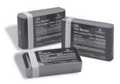
Self-contained, highly intumescent pillows are designed to firestop a wide variety of through-penetrations including cable trays, conduit and blank openings. Interlocking strips hold pillows securely together yet release easily for retrofit or reuse—just remove and replace pillows as needed.
